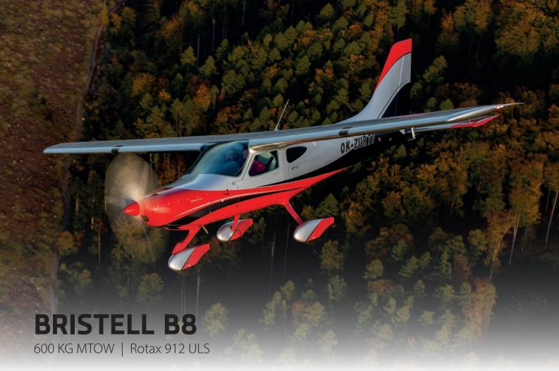
BRISTELL B8 is an all-metal high-wing without struts and with a steerable nose wheel. The cockpit is 125cm wide. The doors of the cockpit as well as the luggage compartment door are made from composite material.
