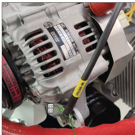
Bonding of the external alternator - alternator bonding cable drawing 34B220203N - cable installation drawing 34B220204N
