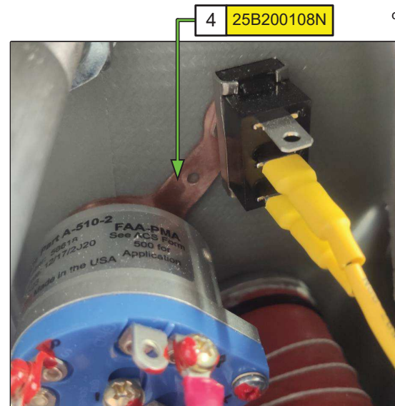
Wire used for interconnecting copper plates M22759/16-12-0
