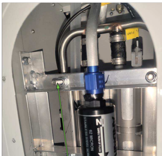
Bonding of the fuel pump - The fuel pump is bolted to the aluminium console which is attached with bolts to the aircraft structure.
