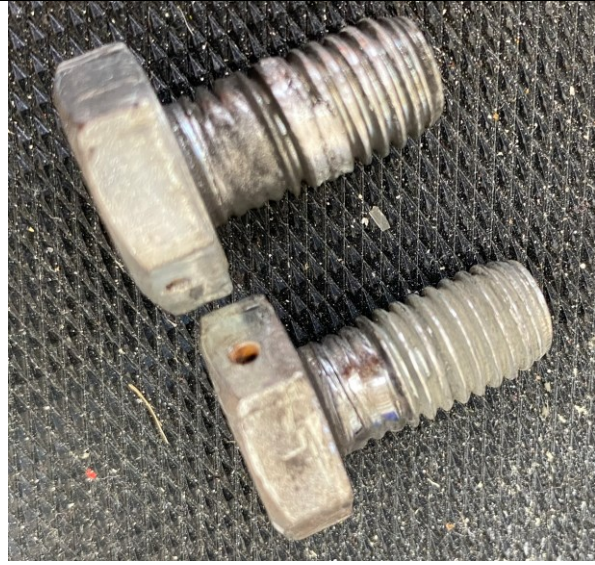
Figure 3 Bolts showing wear on thread
