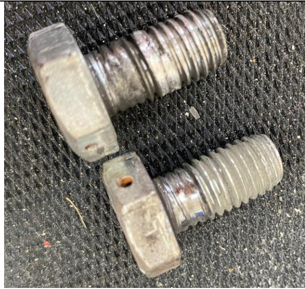
Figure 3 Bolts showing wear on thread
