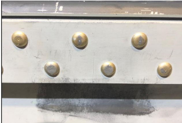
Figure 1: Observed wear on main spar rivet heads and web.
