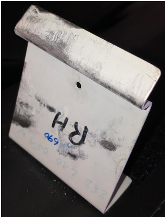
Figure 2: Observed wear on seat bracket (25B210051N, dismantled)
